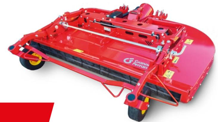
**Blade transmission** by mechanical reducers with spheroidal cast iron boxes and helical bevel gears in an oil bath **is robust and reliable**. The discs with **shockproof swing back blades** protect the transmission against impact with foreign objects left in the grass.
