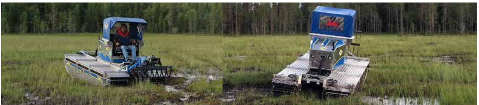
The weight distribution system gives low ground pressure and floating capacity to the machine, offering unique opportunities for work in sensitive environments.
