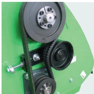
Facile tensione cinghie. Easy belts tightening adjustment.
